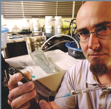
A Georgia Tech researcher displays a prototype of a scanner that uses ultrasound to help medical personnel locate veins.
