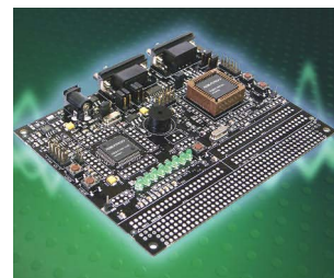
A new, low-cost evaluation kit from Ramtron offers a hardware- and software-design environment for 8051-microcontroller projects
