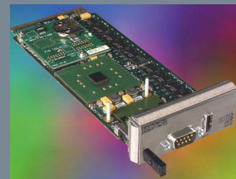
Concurrent Technologies' single-width, full-height AdvancedMC processor module incorporates Intel's 2-GHz Pentium M processor.
