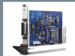
The PXI-3488 interface-controller card offers test-and-measurement-equipment designers a high-speed option for PXI modular-instrumentation systems.
